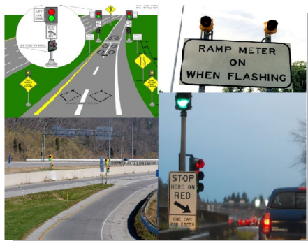
Ramp Metering System: Simulated and Actual
